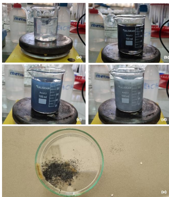
Figure 3.2 Silver nitrate solution (a), Solution with added GO (b), Solution after adding KCl (c,d), Final product Ag/AgCl@GO (e).
