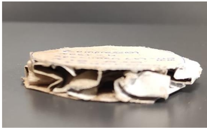
Figure 2.6. Fully crushed circular honeycomb specimen.
