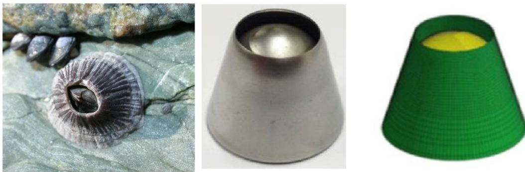
Figure 1.3. Balanus, Balanus-shaped core sandwich structure specimen and FE model 8 .
