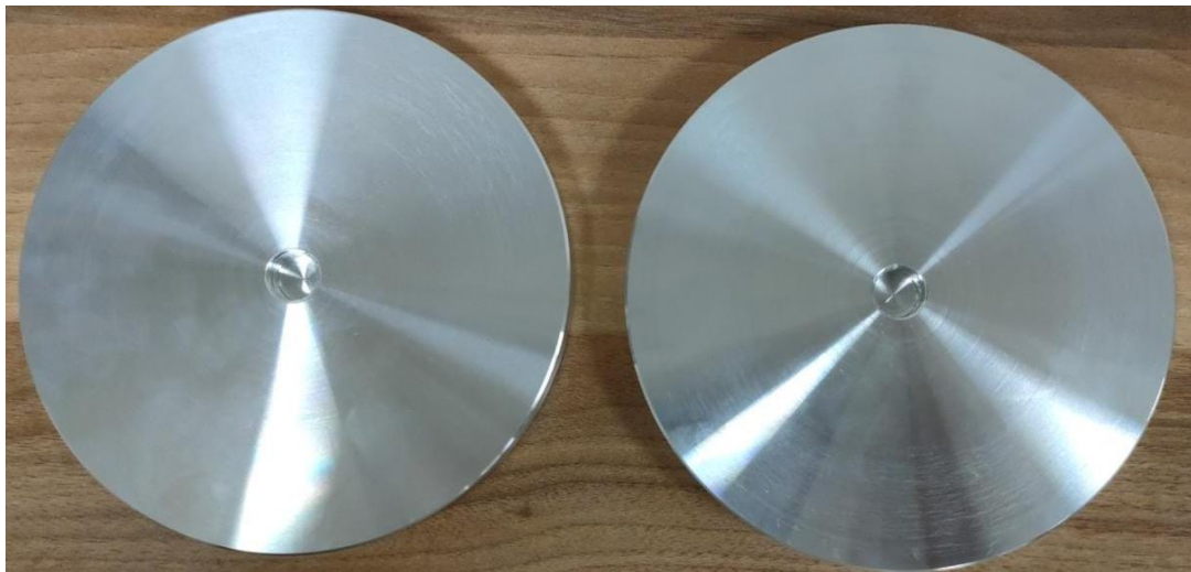
Figure 2.5. Top and bottom compression test plates of Shimadzu AG-X universal testing machine.
