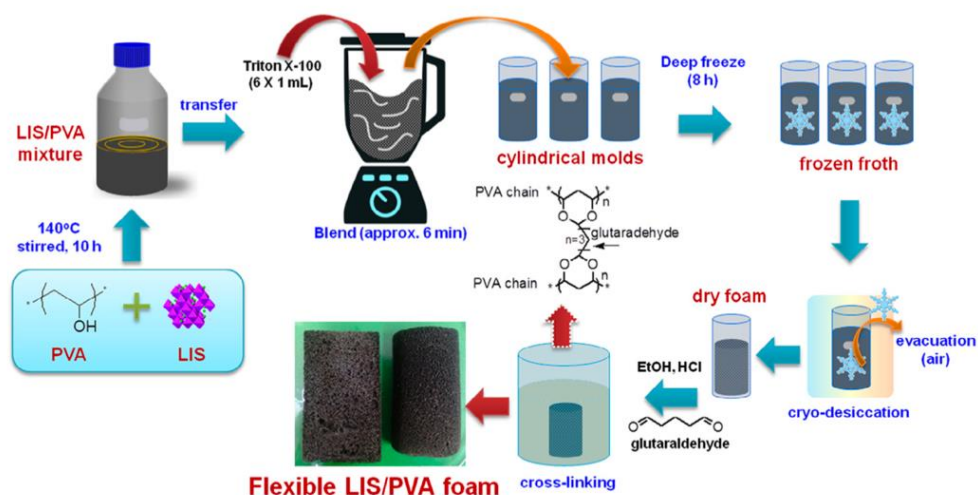
Figure 11. LIS/PVA foam preparation with surfactant blending and cryo-desiccation combination in schematic diagram
