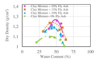
Figure 4 Dry density (g/cm<sup>3</sup>) versus water content (%) for (1) C+0% FA, (2) C+10% FA, (3) C+15% FA, and (4) C+20% FA
