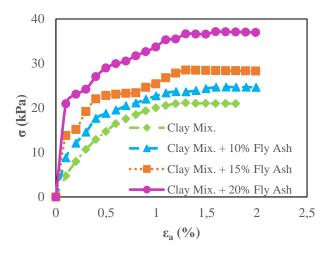
Figure 7 Stress ( $\sigma$ , kPa) versus axial strain ( $\epsilon_a$ , %) graph obtained from UCS tests
