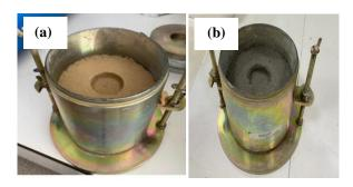
Figure 8 California Bearing Ratio (CBR) Test: (a) clay mixture + 0% fly ash; specimen after penetration, (b) clay mixture + 15% fly ash; specimen after penetration
