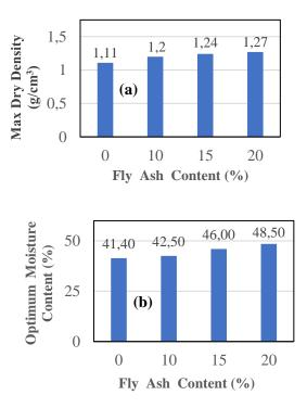
Figure 5 (a) The variation of maximum dry density (g/cm<sup>3</sup>) with fly ash content (%), (b) the variation of optimum moisture content (%) with fly ash content (%)
