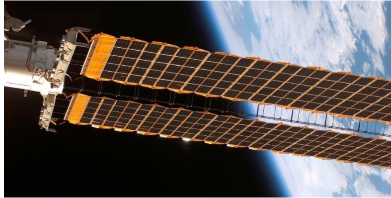
Figure 2.5. Solar array wing panels on the International Space Station deployed and supported by the FAST Mast (Source: NASA)
