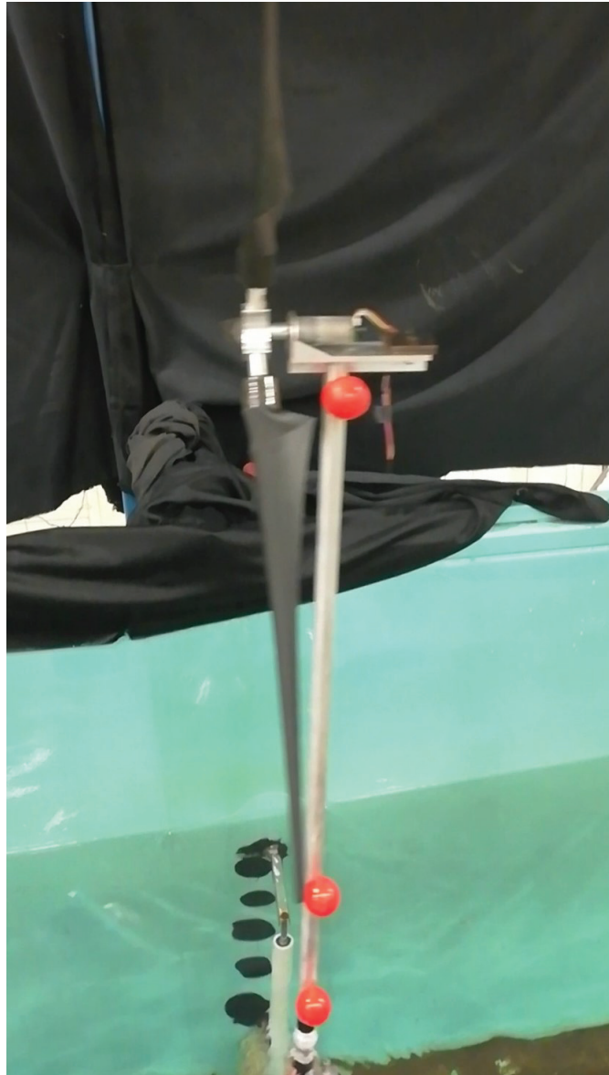
Figure 4.11. Ping-pong balls that placed on the tower
