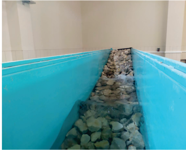
Figure 4.2. The dissipating beach with 1/5 gradient placed at the end of the channel
