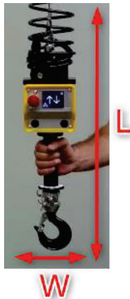
Figure 14: Example of electrical physical human-robot interface (Source: Indeva Intelligent Devices for Handling, 2022)
