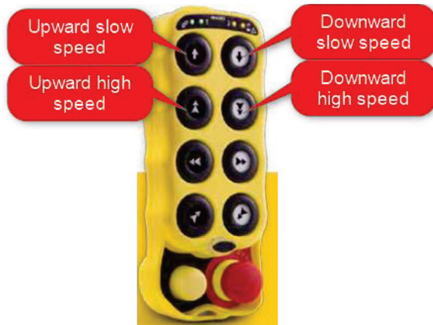
Figure 2: Example of a crane remote controller. (Source: GURALP Crane and Machinery, 2017)
