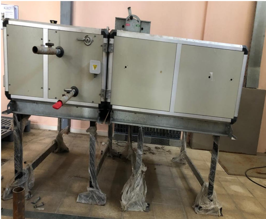
Figure 4.5. The feet of the dryer are mounted and the cabinets are connected to each other
