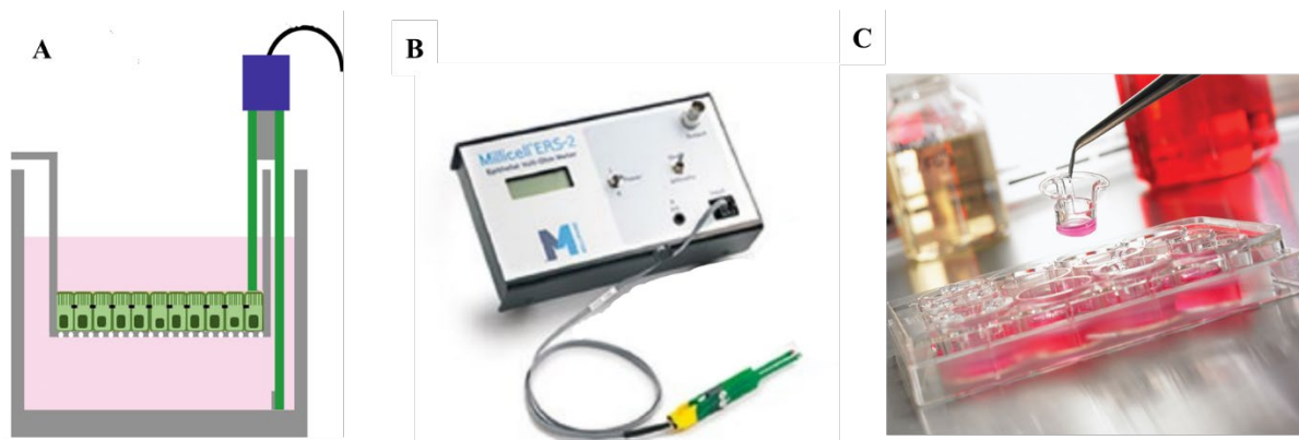
Figure 2.3. Transepithelial Electrical Resistance (TEER) Measurement; (A) TEER is measured by replacing the short electrode in the medium in the upper chamber while the long electrode is placed into the medium in the lower chamber. (B) EVOM device. (C) 12-well insert wells.
