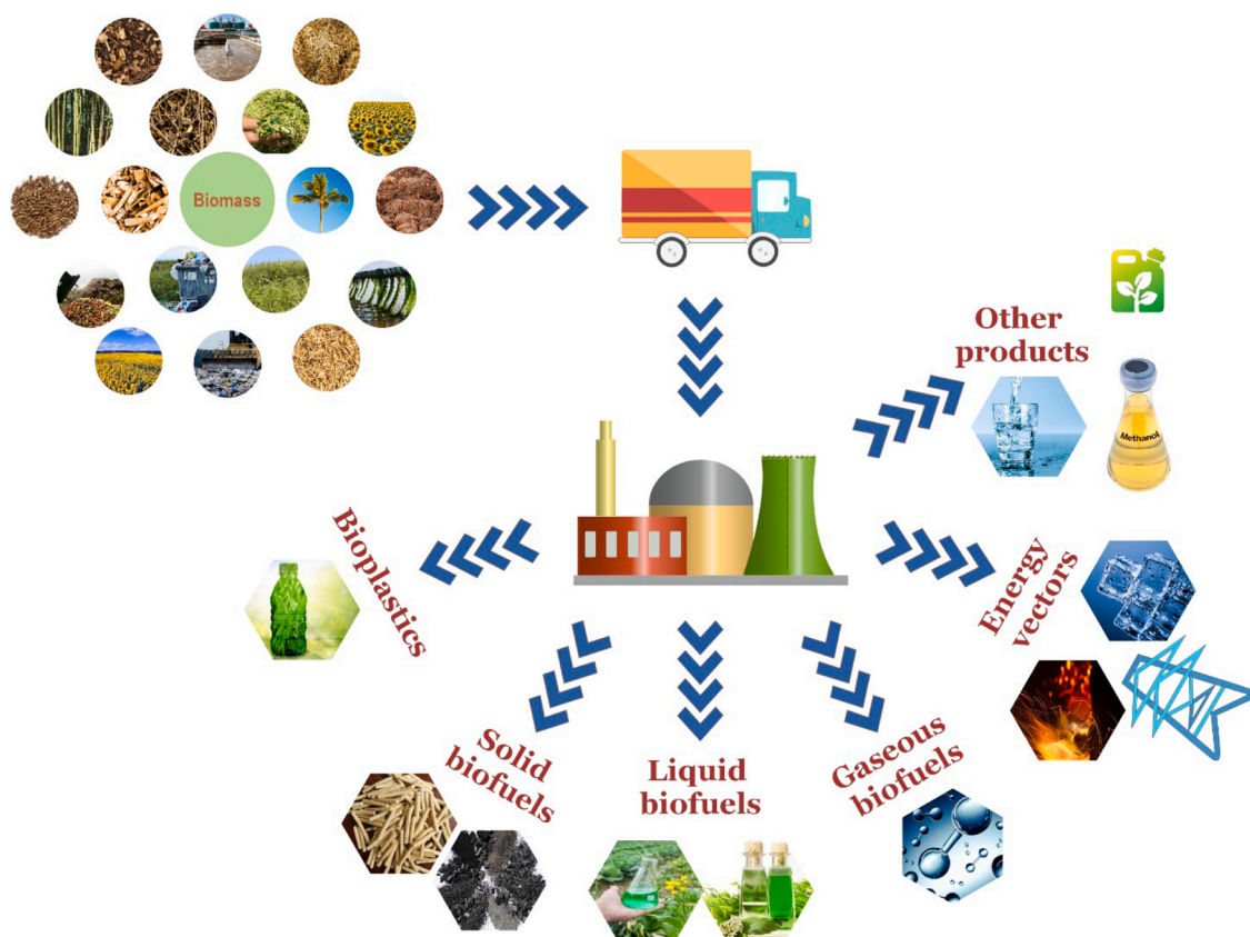
Fig. 1. Schematic diagram of the biomass-based polygeneration system.
