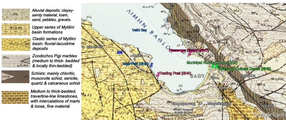
Fig. 32 Detail of the geological map of Samos, according to the Hellenic Survey of Geology and Mineral Exploration (HSGME 2020). A number of boreholes are shown, carried out on the same geological formation (al2)
