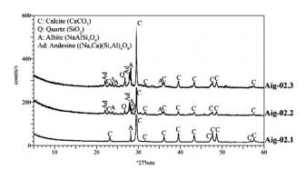
Figure 6: XRD patterns of the Aigai samples show the differences due to a different aggregate usage
