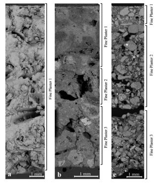
**Figure 3:** SEM images of the cross-sections of plaster samples from: a) Anaia (An3), b) Olympos (O1), c)Aigai (Aig4)
