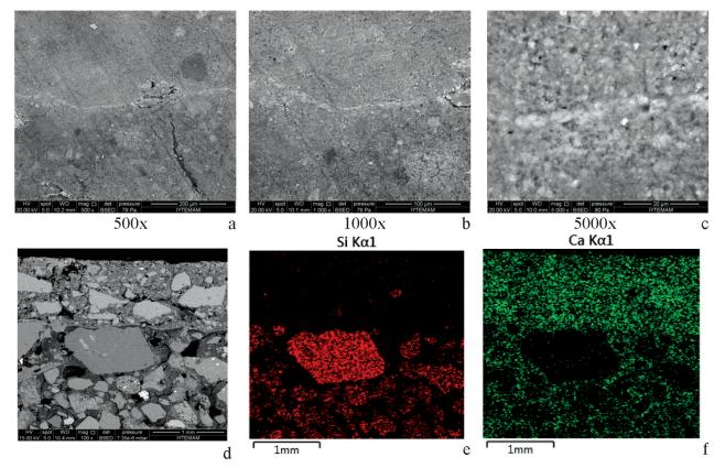
Figure 4: a, b, c) SEM images of the interface of the successive fine plaster layers (O1) from Baspinar, d) SEM image of the polished section of marmorino and intonachino layers (Aig2), e) elemental mapping (Si) of marmorino and intonachino layers of Aig2, f) elemental mapping (Ca) of marmorino and intonachino layers of Aig2
