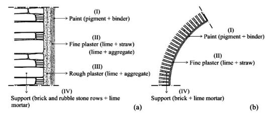
Figure 2: Schematic sections of the wall paintings: a) walls of the Baspinar Church, b) vault of the substructure of the Anaia Church
