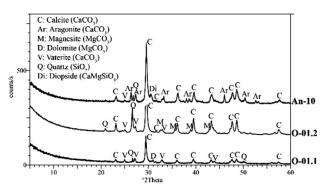
**Figure 5:** XRD patterns of the Olympos and Anaia samples display different polymorphs of CaCO<sub>3</sub> (calcite, vaterite, aragonite) formed with the recrystallization of dissolved calcite due to the wet-dry cycle in the humid atmosphere
