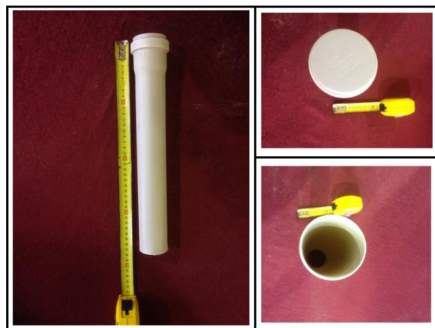
Figure 4.1. PVC pipe model and its cap used in the physical model
