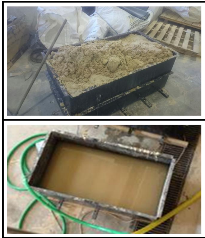
Figure 3.28. Soil preparation boxes
