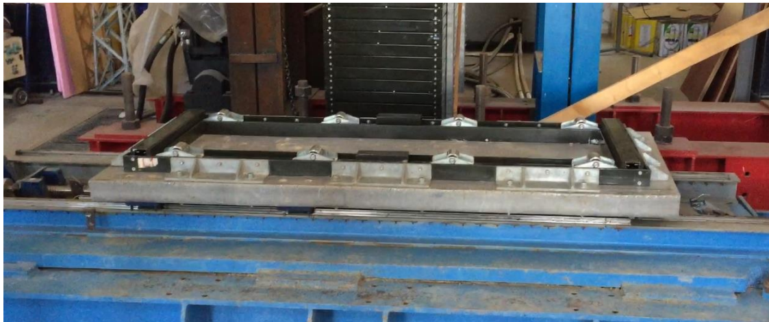
Figure 3.6. Shake Table and first laminate mounted to shake table
