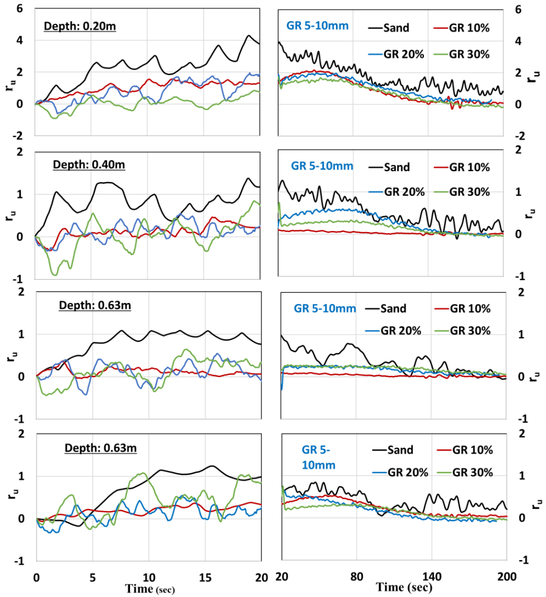
Figure 3.42. Pore water ratio of the tests performed with 5-10mm GR
