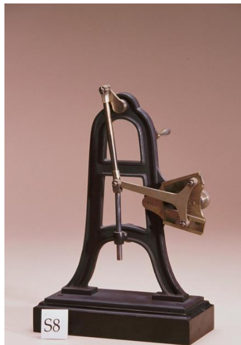
Figure 2.5. Robert's straight-line mechanism from Reuleaux's Collection in Cornell University (Source: ASME, 2004)
