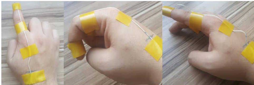
Figure 47: Cable slack after finger flexion and extension.
