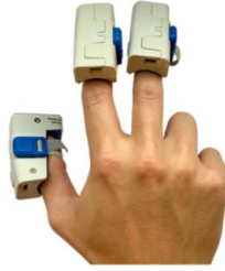
Figure 14: VRtouch Thimble Modules
