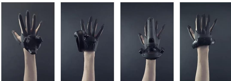
Figure 20: Plexus with Vive Tracker (a), Oculus Touch (b), Vive Controller (c) and Windows VR Controller (d) (Source: Plexus, 2021)
