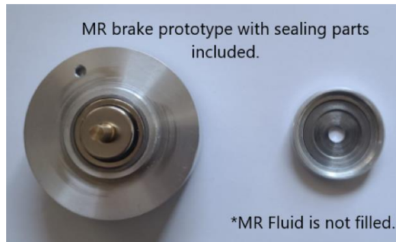
Figure 82: MR Brake prototype without MR fluid.
