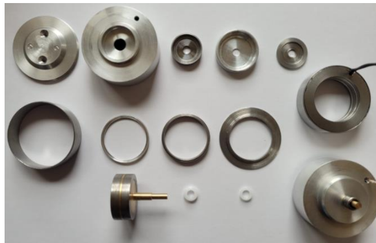
Figure 77: Manufactured and assembled MR brake parts.
