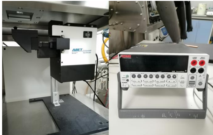
Figure 4.8. Abet 11002 SunLite solar simulator and Keithley 2400 source meter.
