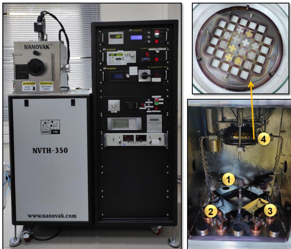
Figure 3.3. The NVTH-350 thermal evaporation system in quantum device laboratory. The chamber includes (1) tungsten wire basket for evaporation of SiO, (2) chromium plated tungsten rod, (3) tungsten boat for evaporation of Au, (4) substrates placed in the sample holder are held inverted at the top of the vacuum chamber.
