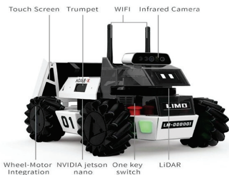
(b) Samples from the ,"Limo", which is the customizable mobile robot product of AgileX [2].
