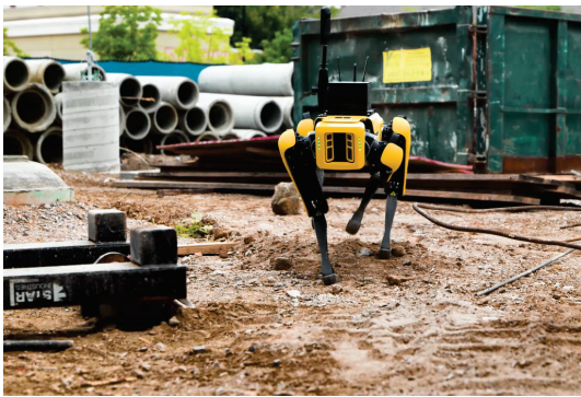
(a) Samples from the product of Boston Dynamics , "Spot", designed for construction industry [3].
