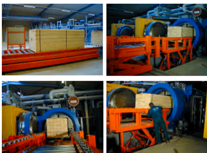
Fig. 13. The world's first commercial supercritical wood treatment plant: receiving and handling system [159].
