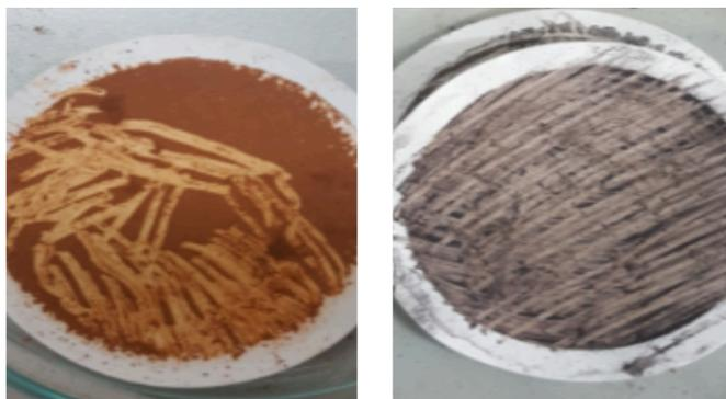
Fig. 2. Sb-rich precipitates obtained artificially in the lab 2 h and 12 h reaction time on filter paper.
