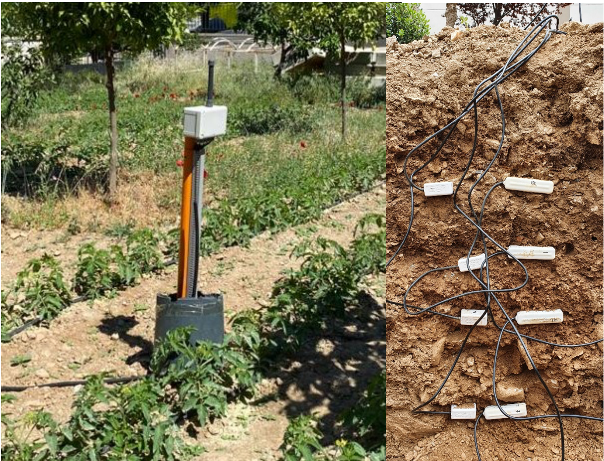
Figure 7. General view of wireless sensor network soil monitoring node (left) and Teros-10 and Teros-12 sensors (right) for tomato production.
