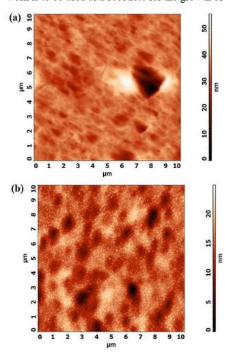
Figure 5 Atomic force microscopy images of (a) asgrown and (b) polished (E5) samples
