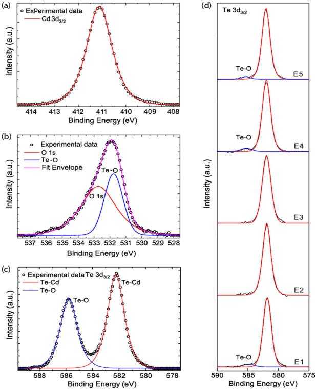
Figure 3 XPS results of (a) Cd-3d3/2, (b) O-1s, and (c) Te-3d3/2 scan of the as-grown CdTe sample. Black dots are experimental data while the continuous red and blue lines are the fit curves. (d) Te-3d3/2 scan of the wet chemically polished CdTe surfaces
