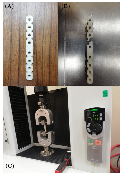
Fig. 4 (A) Production of students’ designs with a 3D printer, (B) failure as a result of applying the tensile test, (C) performing the test by Shimadzu Tester.
