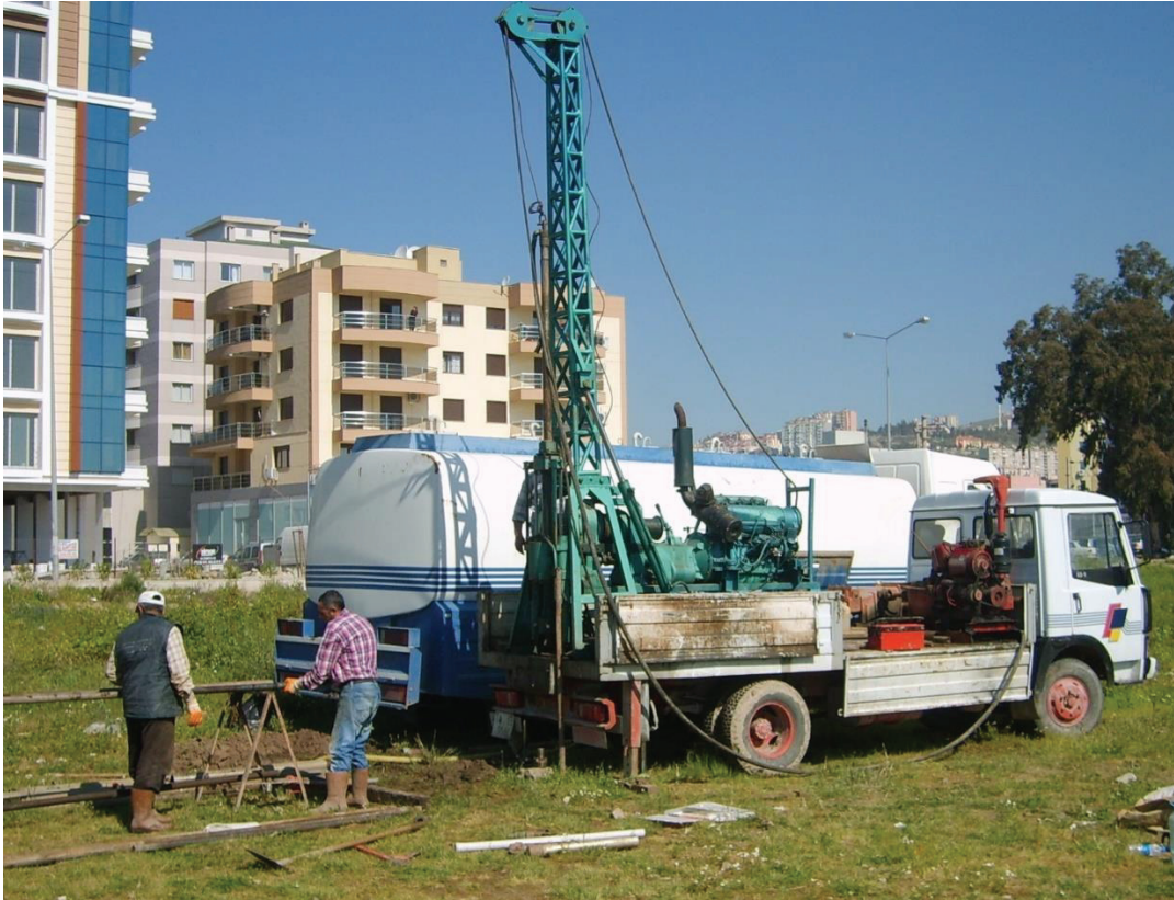
Figure 3.1. The photo of SPT test truck and SPT tests application in the region between Cigli and Karsiyaka taken by Ecemis et al.
