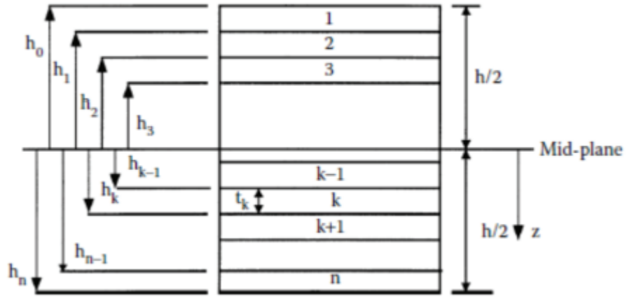
Figure 3.3. Schematic representation of a symmetric laminate (Source: Kaw 2006)
