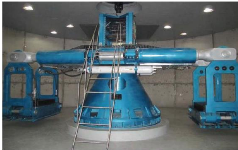
Figure 2.4. Centrifuge setup (Source: Huang et al., 2014).
