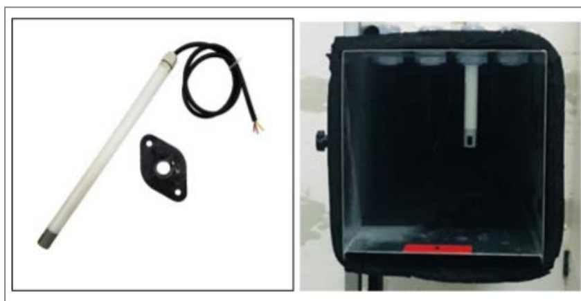
Figure 3.16. Blitz Sens VS-C2-1-A air velocity transmitter and in-channel measurement
