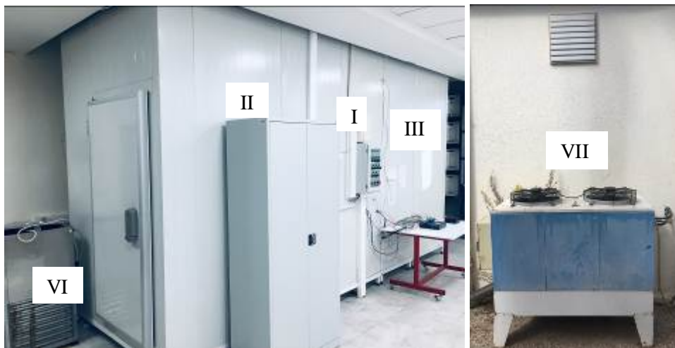
Figure 3.1. The experimental setup; I: aerated concrete wall, II: indoor environment, III: outdoor environment, VI: constant temperature bath, VII: cooling group.
