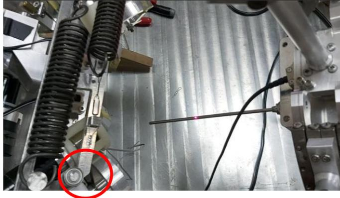
Figure 38: Bearing added on the pin
