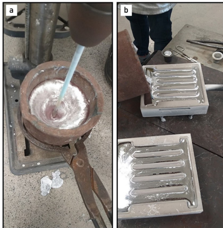
Figure 3.5. (a) Casting of Sc-A356 Alloy, (b) Casting alloys into molds for tensile testing.
