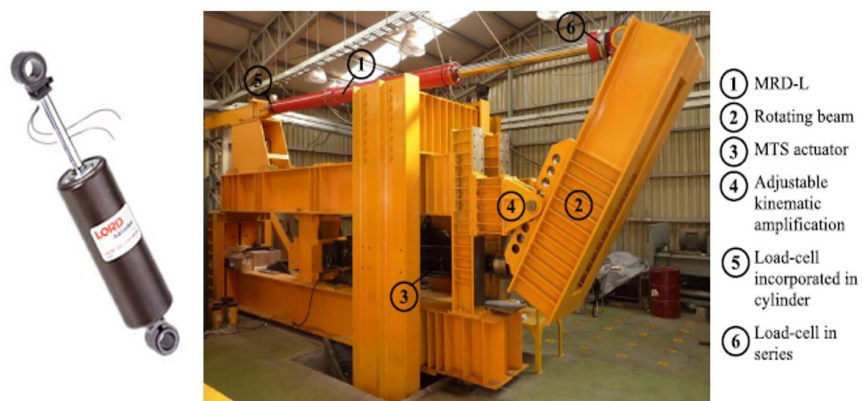
Figure 2.8. RD 1005-3 MRD (Produced by LORD Corp.) and the long-stroke MRD (Source: Zemp et al. (2016))
