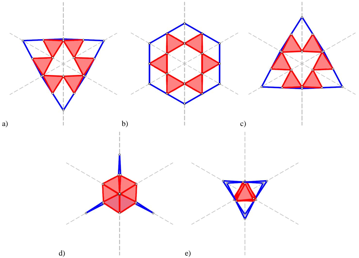
**Figure 9** 5 configurations of a hexagonal closed loop rhombus assembly with V-type connections and TI pattern
