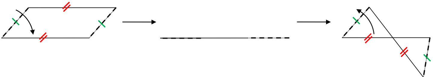
**Figure 6** Assembly mode change of a parallelogram loop into an anti-parallelogram loop through the singular configuration
