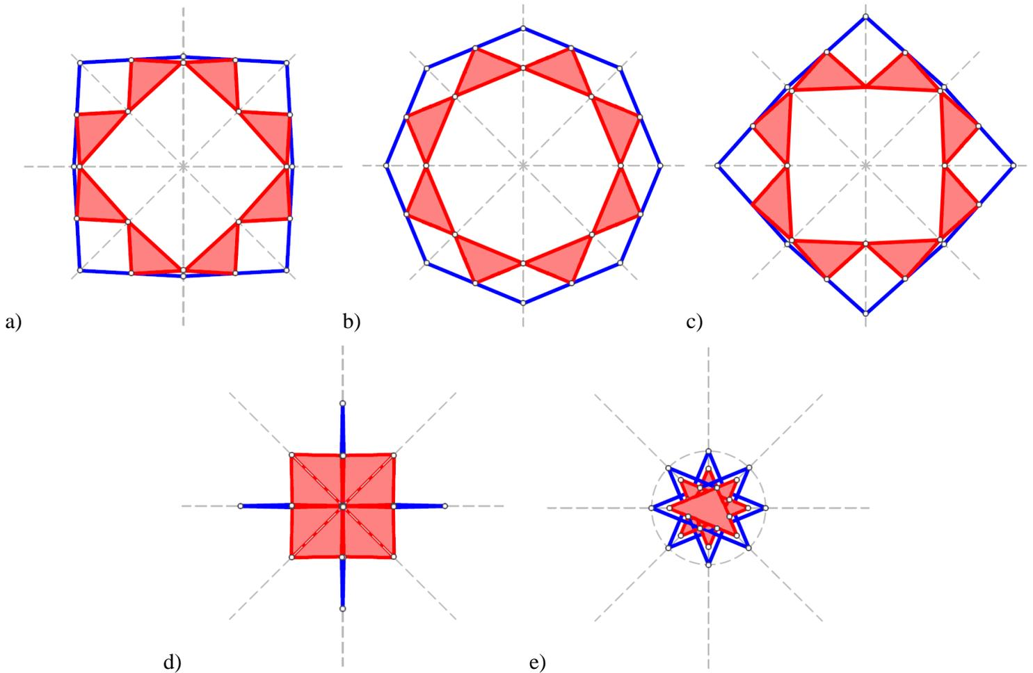
**Figure 10** 5 configurations of an octagonal closed loop rhombus assembly with V-type connections and TI pattern
