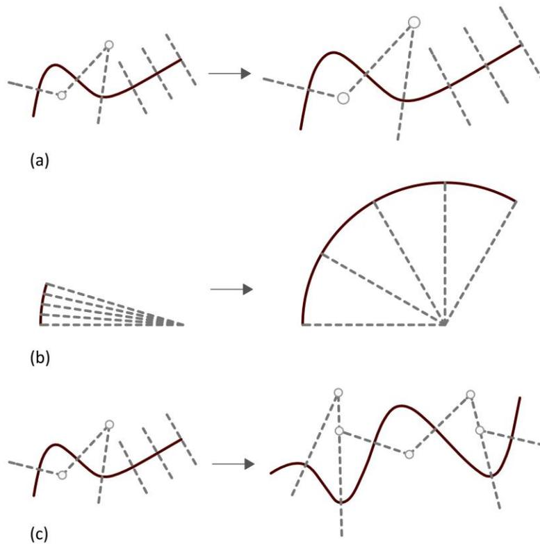
**Figure 2** Deployable vs. transformable motion: a) scaling/dilation type deployable; b) angular deployable; c) transformable [42]
