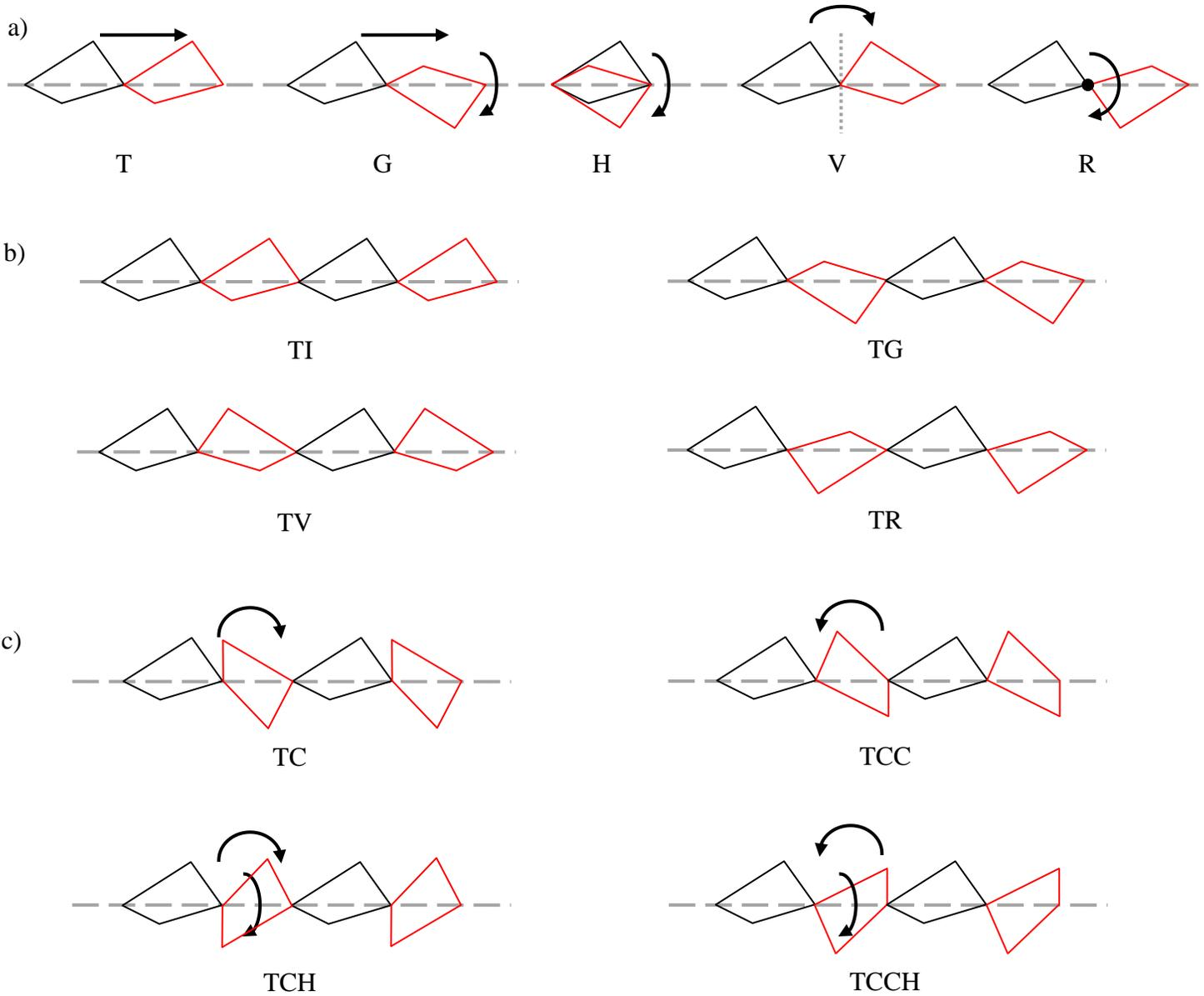
**Figure 8** a) Basic isometry operations, b) the first four frieze patterns, c) long-short diagonal connections
