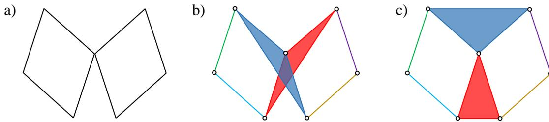
**Figure 7** a) Assembly of two rhombus loops and b, c) 6-link kinematic chains obtained from this assembly by rigidly connecting two pairs of adjacent sides of the loops
