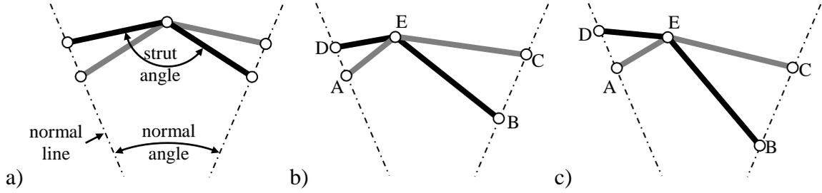
**Figure 1** a) An angulated element pair with equal link lengths and kink angles, b) An equilateral GAE:  $|AE| = |DE|$ ,  $|BE| = |CE|$ ,  $\angle AEC \neq \angle BED$ , c) A similar GAE:  $|AE|/|DE| = |CE|/|BE|$ ,  $\angle AEC = \angle BED$
