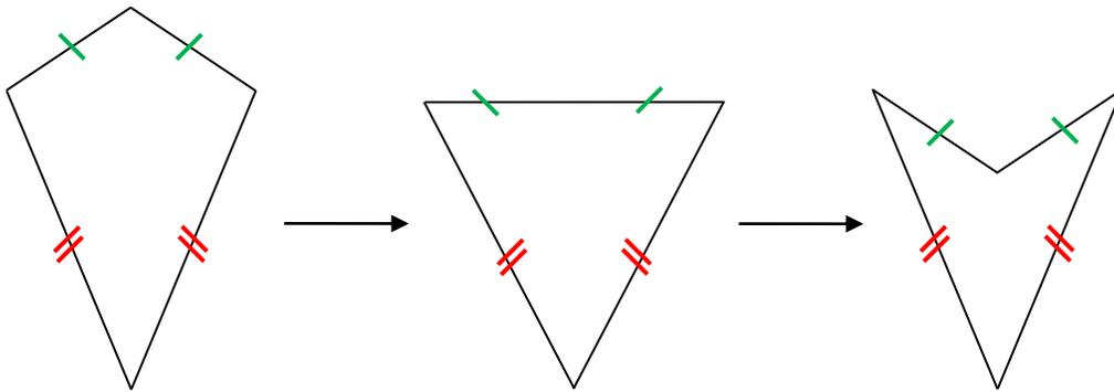
**Figure 5** Assembly mode change of a kite loop into a dart loop through the singular configuration
