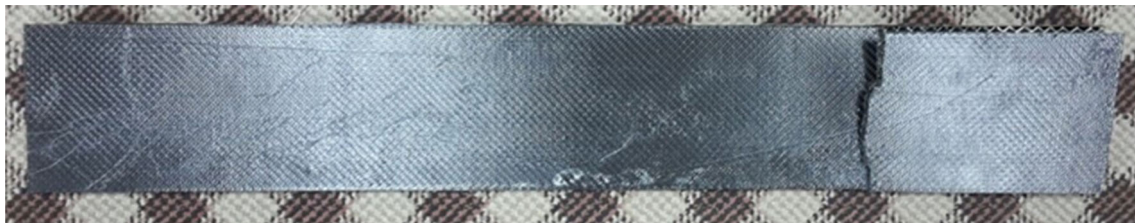
Figure 18. Sandwich beam face fracture.
