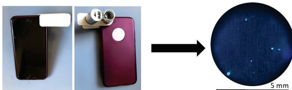
Figure 4.5. Smartphone microscope and an image captured with it.
