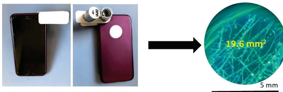
Figure 4.26. Image of the pattern taken by smartphone microscope (60X objective magnification) under 365 nm UV light.
