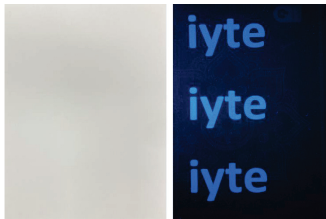
Figure 2.12. The photograph of pattern printed using CDs ink (1% blue luminescent CDs) under visible light and UV light (365 nm).
