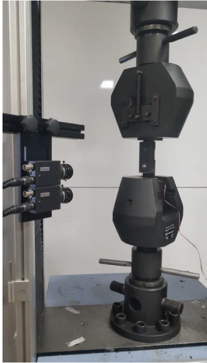
Figure 3.9. Quasi-static bearing test set-up
