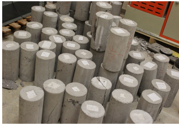
(c) Cylinders after testing
