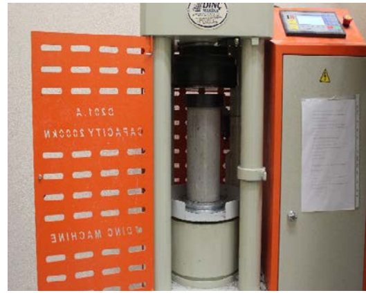
(b) Cylinders placing in machine
