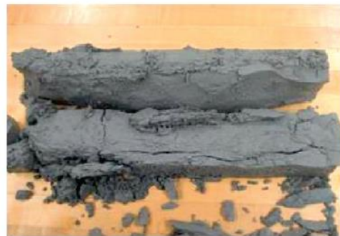
(b) ECC2 matrix (ECC2 w/o fiber) after 60 freezing and thawing cycles
