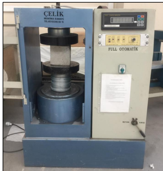
Figure 4.13. Concrete compressive strength testing machine
