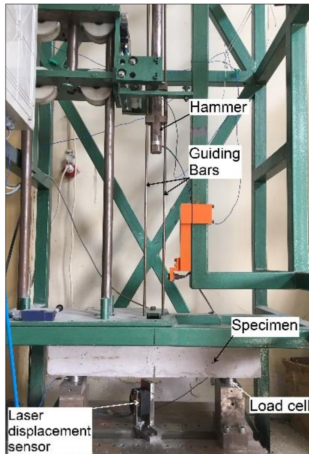
Figure 4.17. Impact loading test
