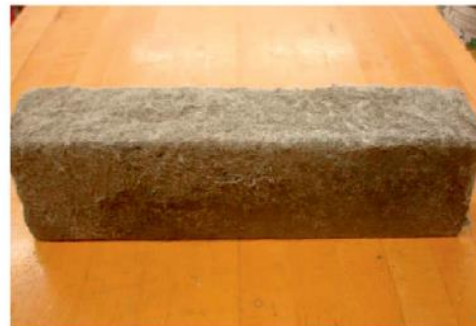
(d) ECC2 after 300 freezing and thawing cycles
