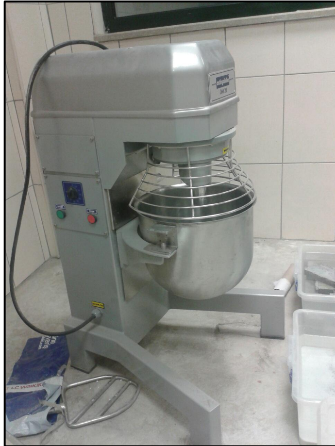
Figure 4.9. 20-liter capacity mixer for ECC production
