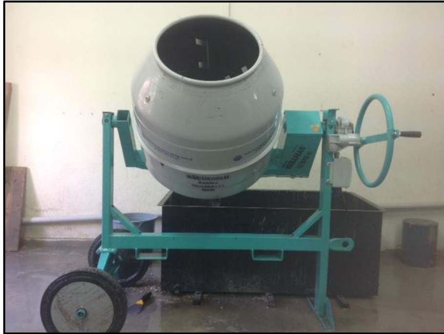
Figure 4.10. Rotating drum mixer with 100-L capacity
