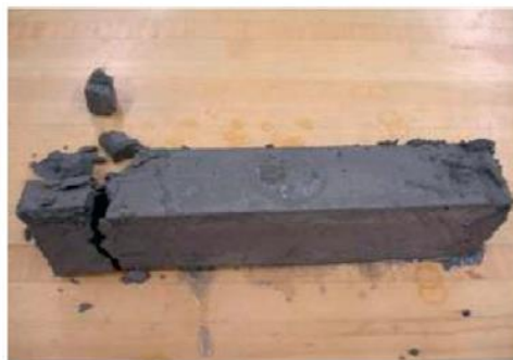
(a) ECC1 matrix (ECC1 w/o fiber) after 210 freezing and thawing cycles
