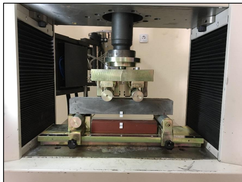
Figure 4.14. ECC mixtures flexural testing
