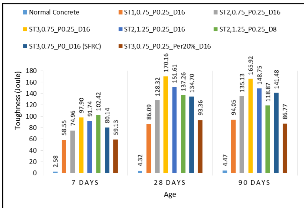
Figure 5.31. 7, 28 and 90 days static bending toughness of selected mixtures
