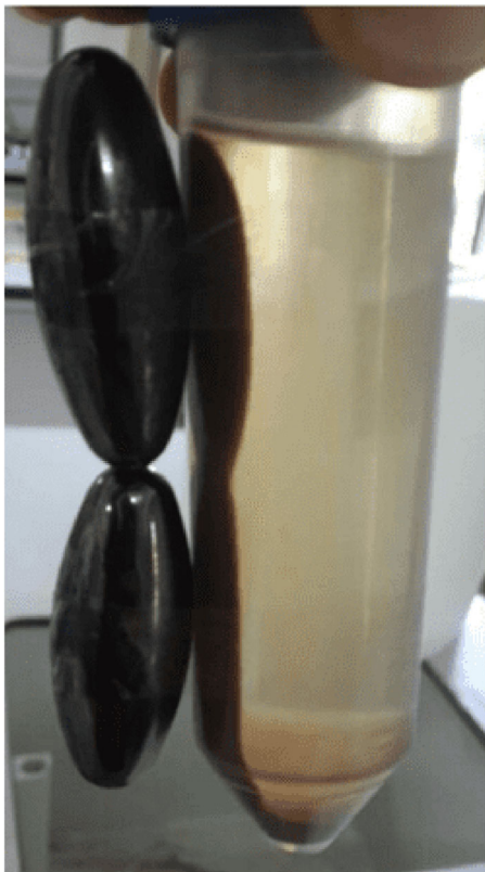
FIGURE 1 Magnetic aggregation of MCNs by magnets
