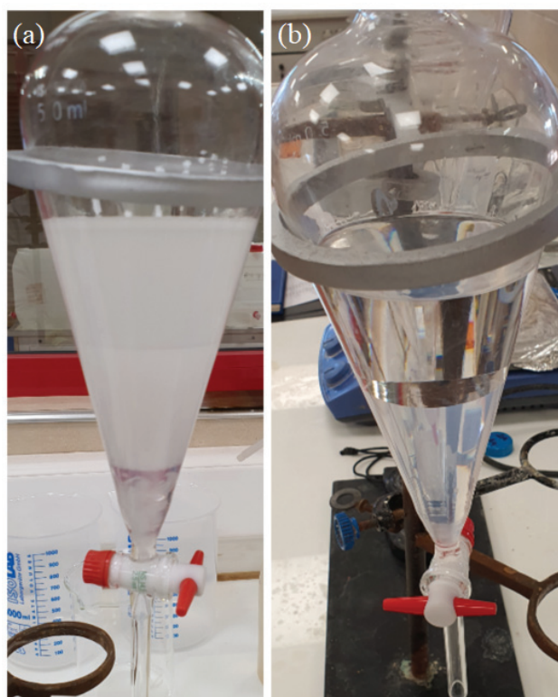
Figure 4. 4. Illustrations of D2EHPA organic phase with NaOH (a) 35% pre-neutralisation (b) phase separation after extraction (c) raffinate phase (d) interface of the organic and raffinate phases
