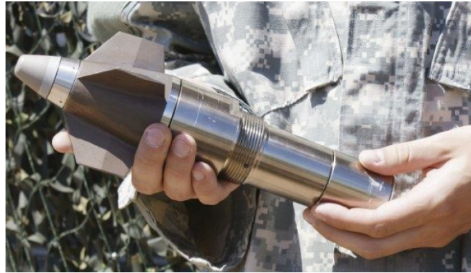
Figure 1.4. M1156 Course Correction Fuse (Source: Mönch Publishing Group (2021))
