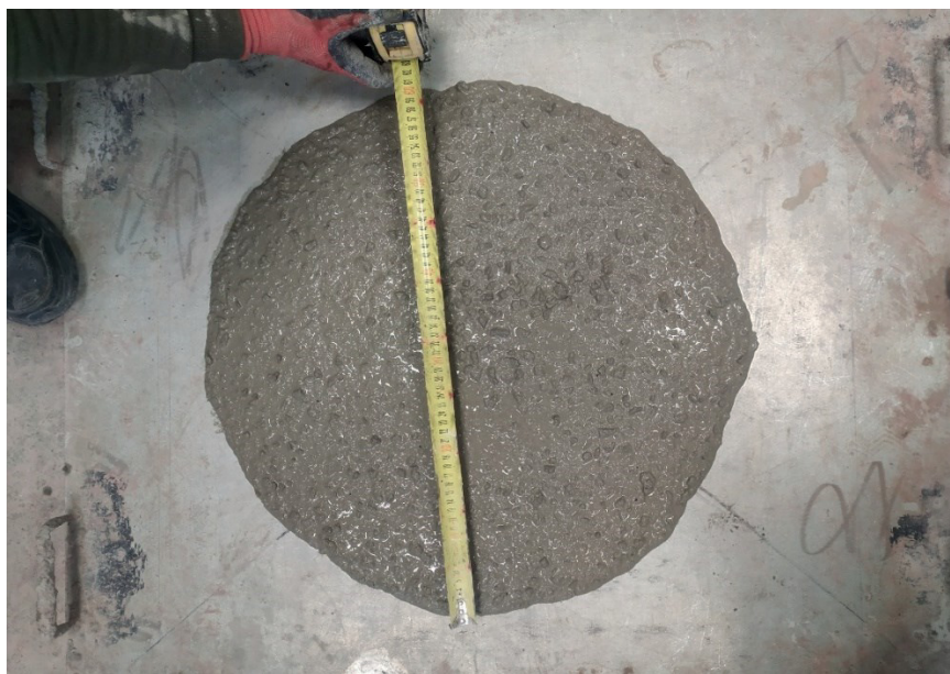
Figure 3.3 Slump Flow Test
