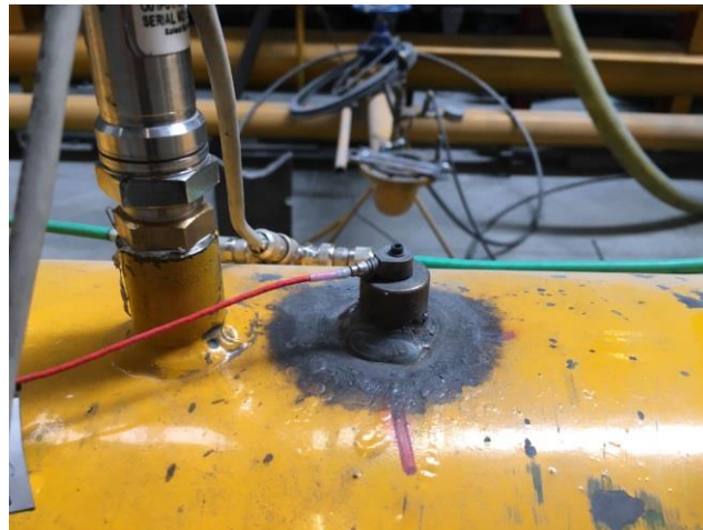
Figure 3.7 CavitationSensing Accelerometer (Endevco, type 7250B-10)
