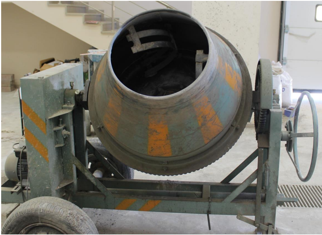
Figure 3.4 Rotating drum mixer
