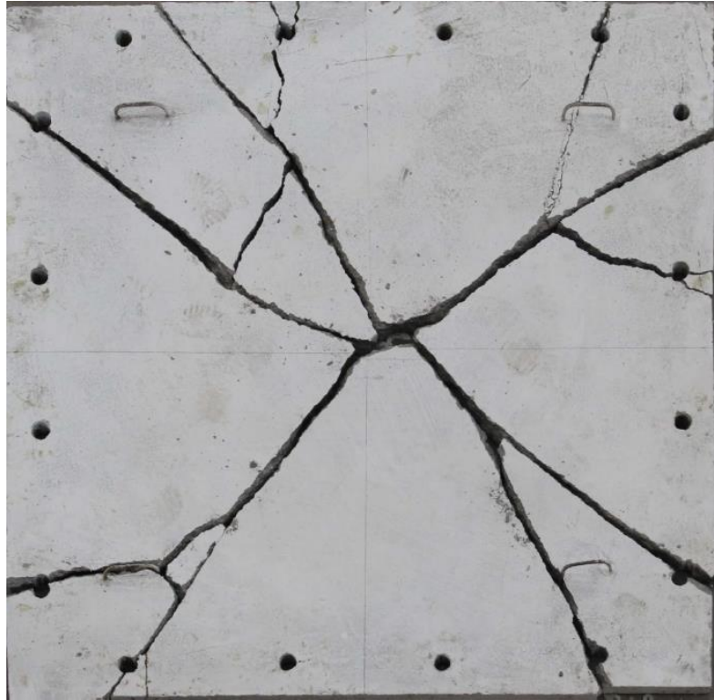
Figure 4.31 JN-plain panel after testing
