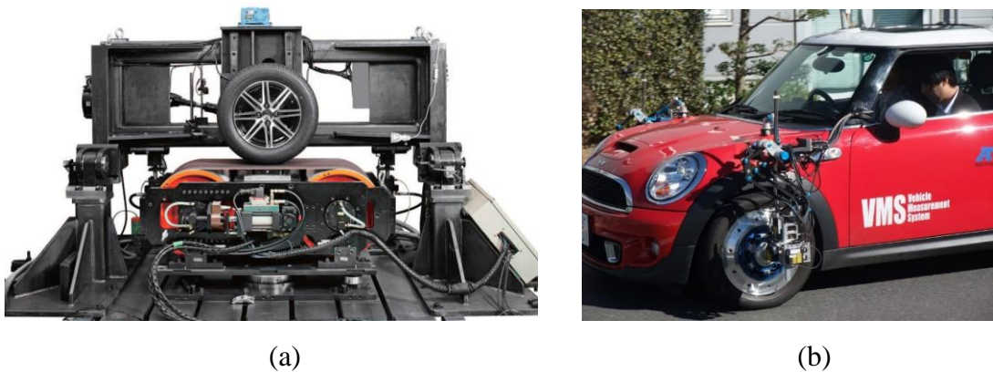
Figure 4.1. Industrial wheel force/moment measurement equipment; a) Flat belt tire test machine b) Vehicle measurement system (Source: A&D Technology, 2020)
