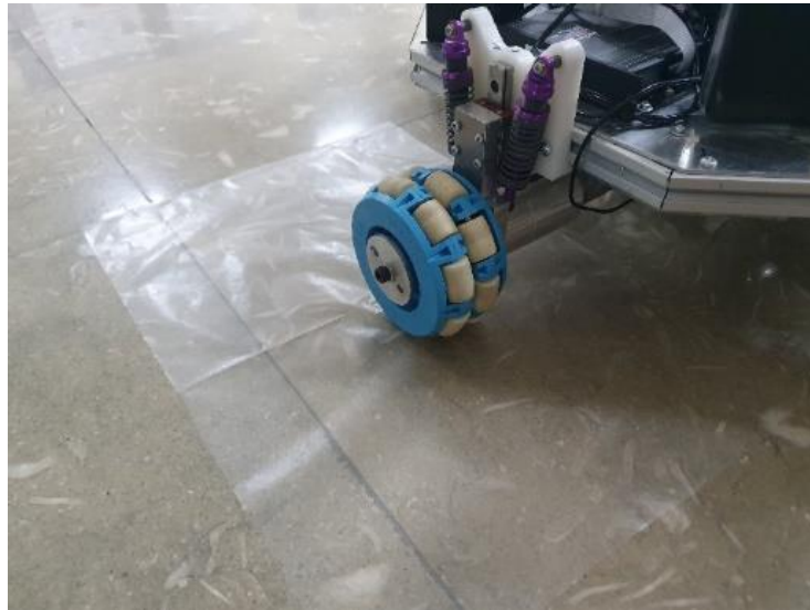
Figure 5.16. Nylon piece placed between UTO wheel and the ground
