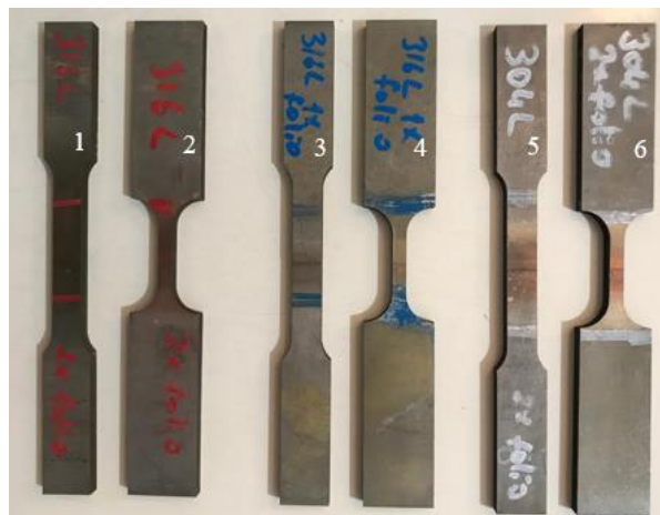
Figure 3.15. Tensile test specimens (1, 3 and 5) and fatigue test specimens (2, 4 and 6)
