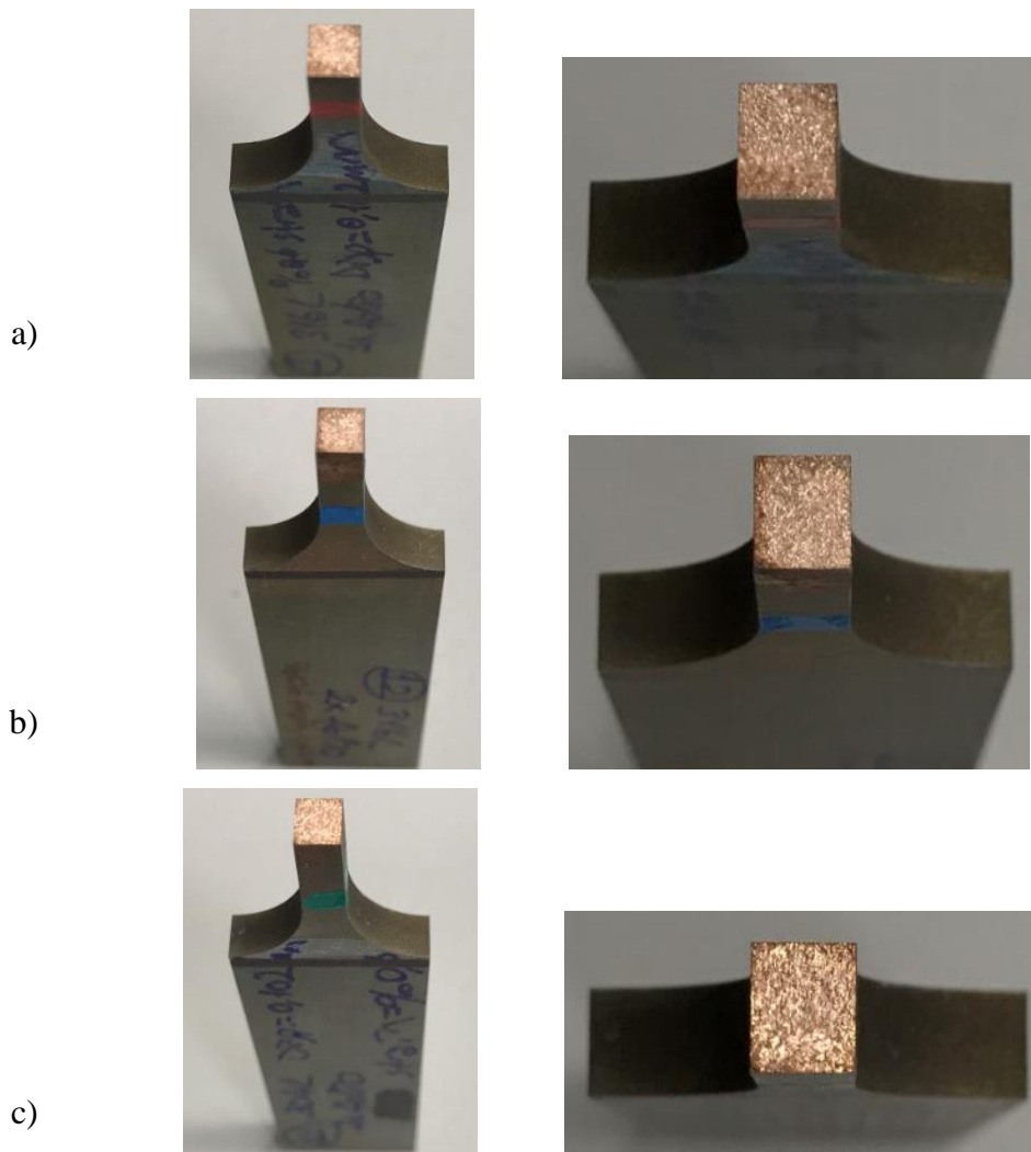
Figure 4.21. Fatigue test specimen fractographs of 316L stainless steel brazed with 50 \mu\text{m} copper (a), 316L stainless steel brazed with 100 \mu\text{m} copper (b) and 304L stainless steel brazed with 100 \mu\text{m} copper (c)
