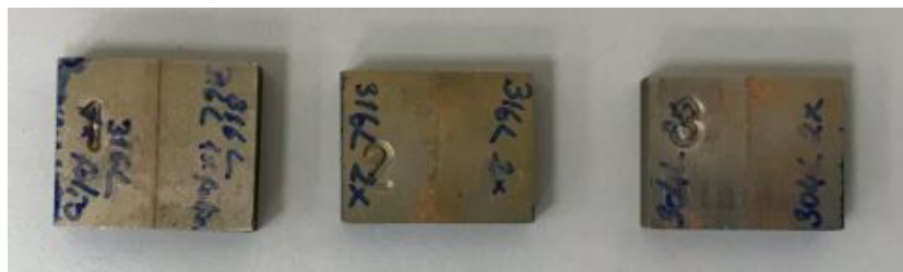
Figure 3.16. Brazed stainless steel coupons
