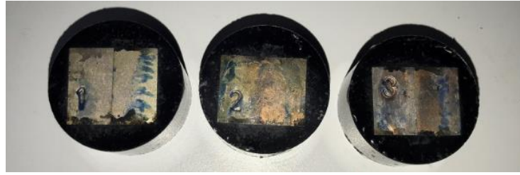
Figure 3.17. Brazed stainless steel coupons from each sample groups inside the hot mounting resin
