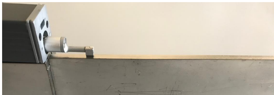
Figure 3.3. Surface roughness measurement of the laser cut stainless steel sheets
