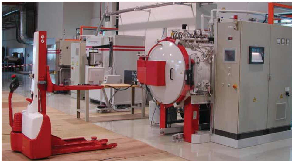
Figure 2.13. Vacuum brazing furnace system [33]
