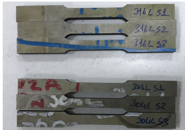
Figure 3.14. Non-brazed 316L and 304L stainless steel tensile test specimens
