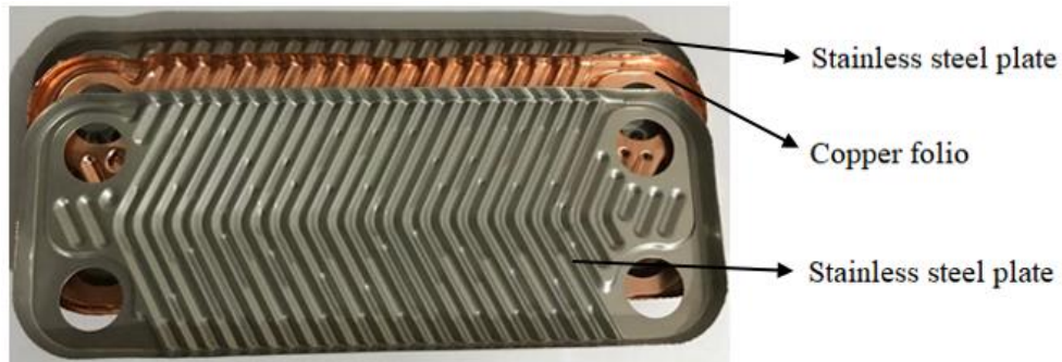
Figure 1.6. Copper foil between two stainless steel channel plates
