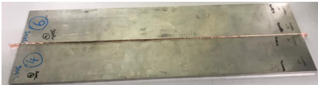
Figure 3.8. Inserted copper foil between two stainless steel sheets before brazing
