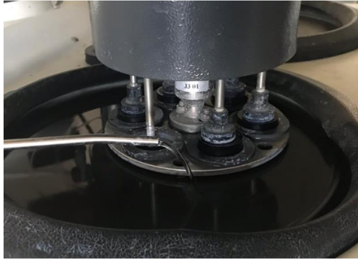
Figure 3.18. Grinding of the samples
