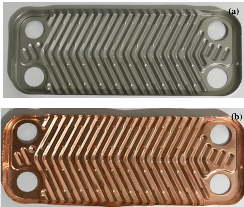
Figure 1.5. Stainless steel channel plate (a) and copper foil as filler material for brazing in production of PHEs for combi boilers (b)
