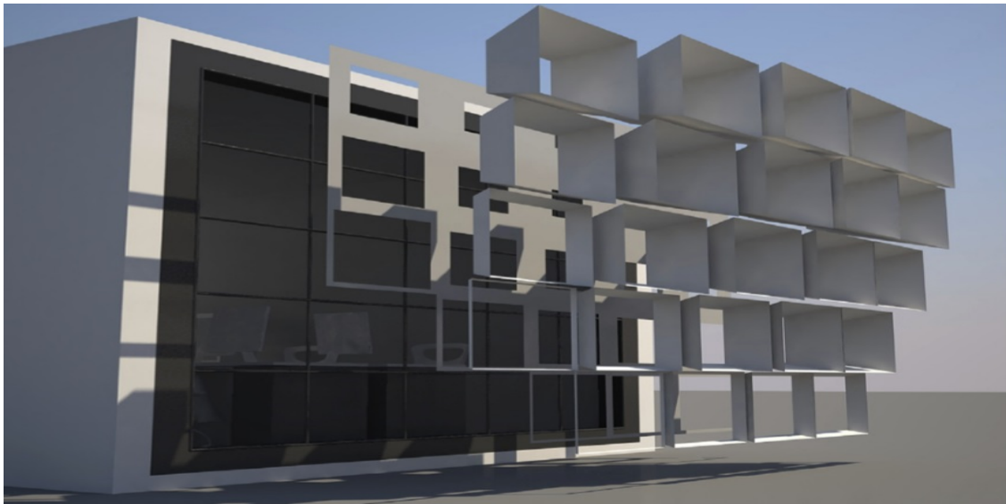
Figure 2.12. Test room model for three cases as a plain window, two-dimensional and three-dimensional shape changes. (Source: Hosseini, Mohammadi and Santin 2019).
