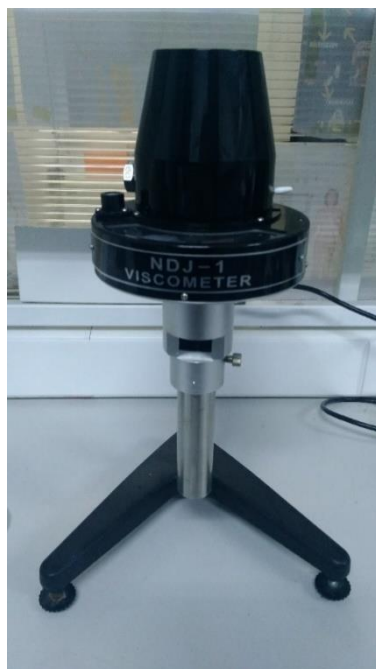
Figure 2.2. The experimental setup for viscosity measurement of precursor inks
