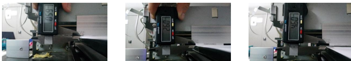
Figure 3.1. Measurement of distance between the inkjet printhead and the tray
