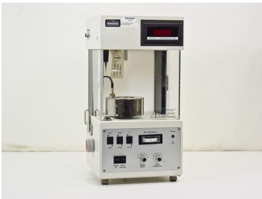
Figure 2.1. The experimental setup for surface tension measurement of precursor inks
