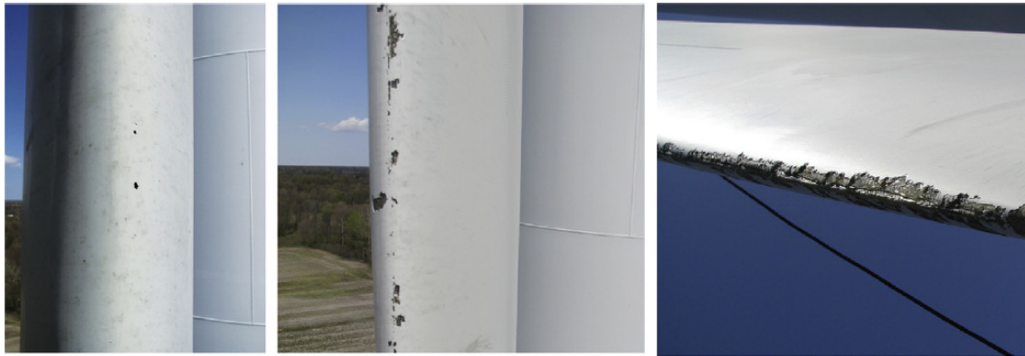
Figure 4.2: Leading Edge Erosion at Several Levels (Source:[van der Mijlemeijer])
