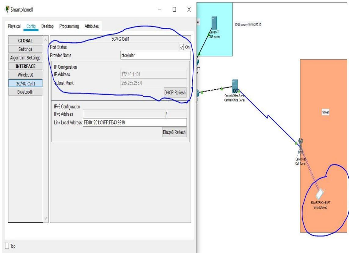
Figure 3.18. Smart Phone Connection to the Cell Tower
