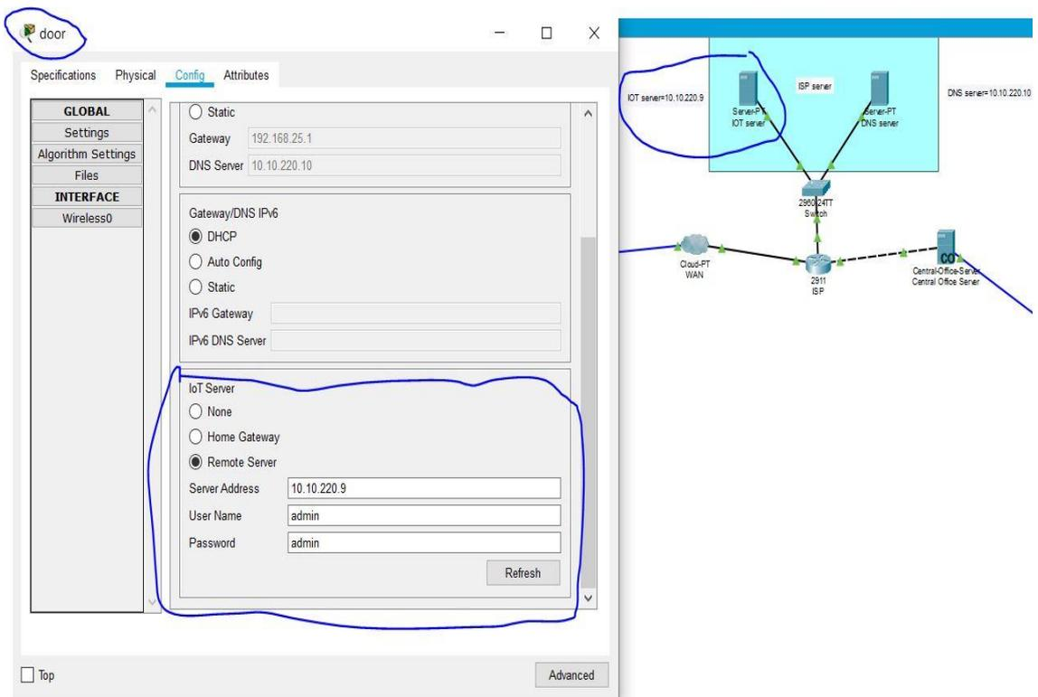
Figure 3.10. Connecting IoT Devices to IoT Server
