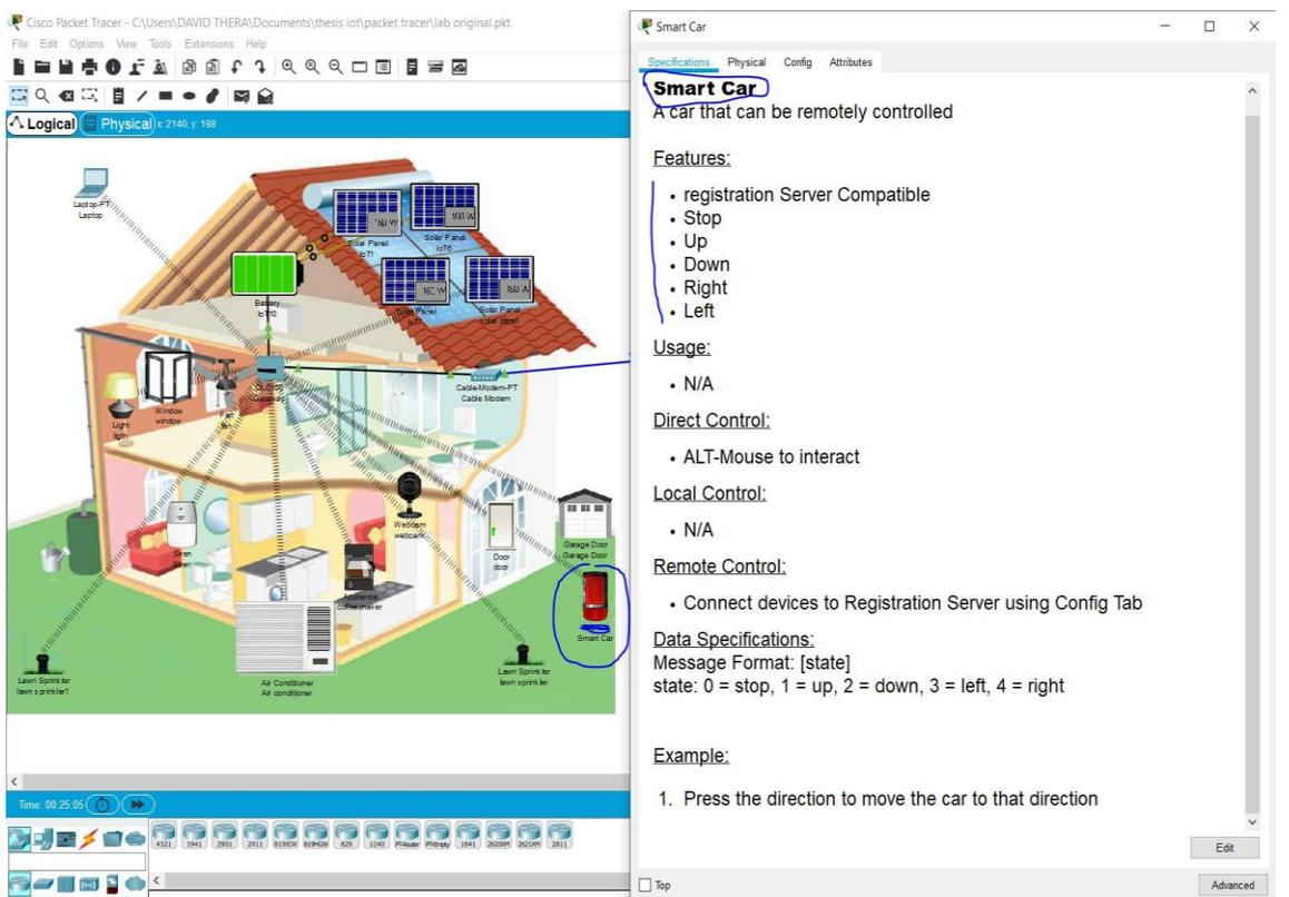
Figure 3.16. Smart Car Specifications
