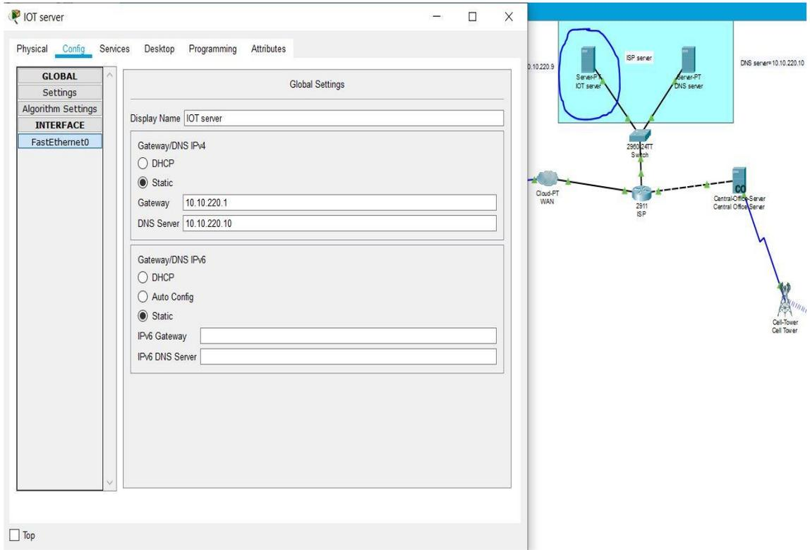
Figure 3.9. IP Address assignment for IoT Server
