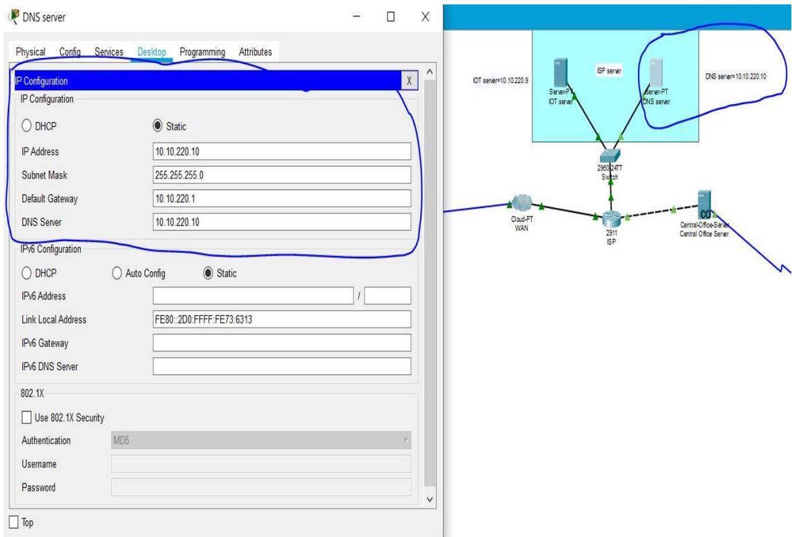
Figure 3.12. IP Address Assignment for DNS Server
