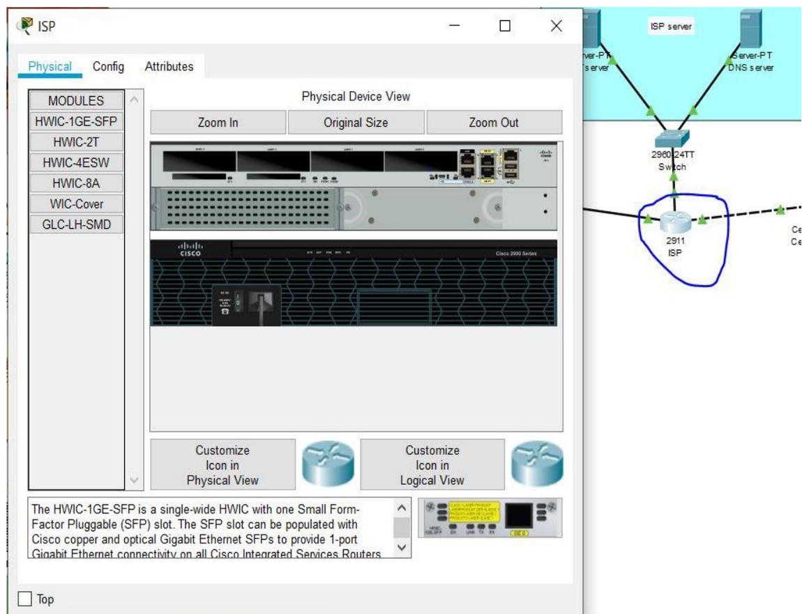
Figure 2.2. Physical View of ISP Router
