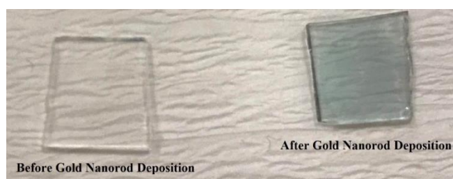
Figure 4.5. Before and after immobilization of GNRs onto glass substrates
