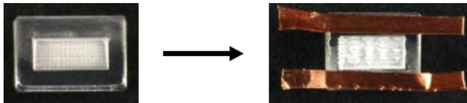
Figure 5. Bare and copper tape functionalized PMMA substrates
